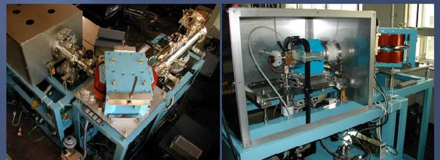
Electron cyclotron frequency  $f_c = 10 \text{ GHz} @ 0.357 \text{ T}$
